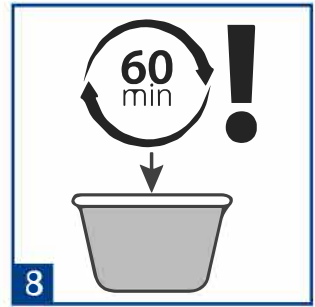
8 Use the mixed tile fix within 60 minutes (from the pot)
